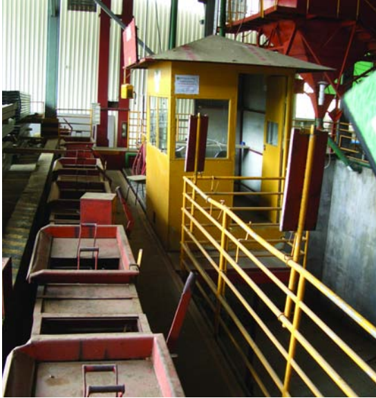
This is the receiving station of the mill at CoopeDota, where farmers deliver their berries. The berries' quality and quantity is determined at this point.
