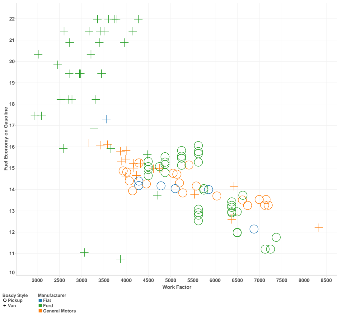
Figure 10-3 Comparison of Fuel Economy and Work Factor for Gasoline Vehicles in the Analysis Fleet
