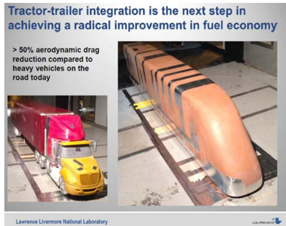
Figure 2-8 Pictures showing future heavy-duty tractor trailer concept to achieve >50% aerodynamic improvement for Class 8 line haul heavy-duty vehicles
