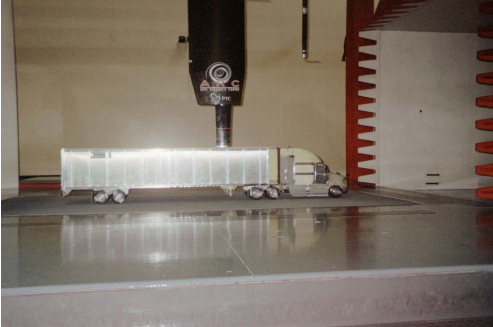
Figure 3-6 1/8th scale tractor-trailer model in ARC reduced scale wind tunnel.
