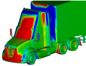
Figure 1: baseline roof fairing
