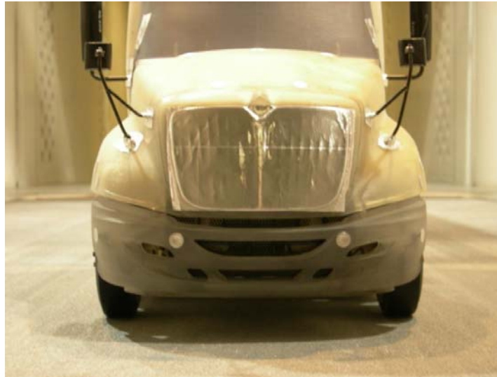
Figure 2-7 Photo of 1/8th scale model of a tractor with the front, external grille covered with aluminum tape to simulate a closed grill configuration.
