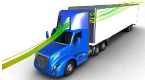
Figure 3: SABIC concept roof fairing showing directed airflow
