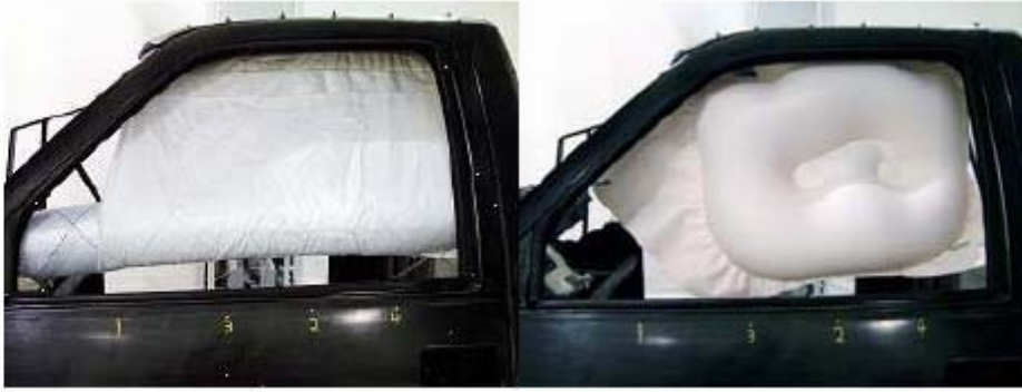
Figure III-6 Prototype Zodiac (left) and TRW (right) air bag curtains on CK pickup.
