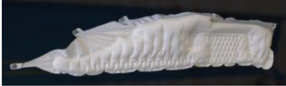
Figure VIII-6B. One-Piece-Woven air bag without tether lines, TRW SHI2
